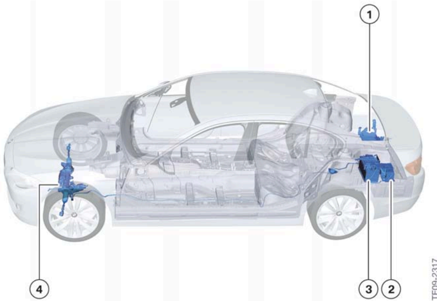
F10 24V components and line routing
